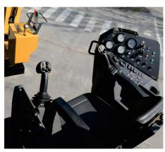
The operator station utilizes ergonomic design, using integrated joystick with fingertip buttons, switches and controls.
