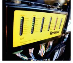
The CAN bus electrical system offers reliable and easy diagnostics.
