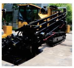
The rack and pinion thrust design offers a reliable and low maintenance power delivery system to helps to improve productivity.
