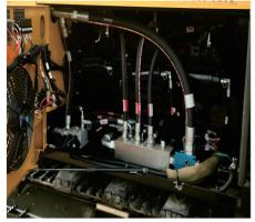
Utilizes a Sauer Danfoss closed loop, variable displacement, piston style hydraulic pump in order to maximize efficiency and reliability.
