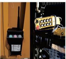
Installed with industry-leading safety features such as remote lockout system, electric strike alert system and operator-presence monitoring.
