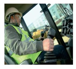
The ergonomically-designed operator station is installed using integrated joystick with fingertip buttons, switches and waterproof controls.
