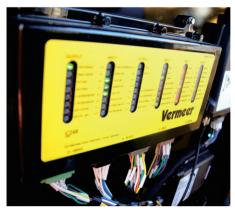
The CAN bus electrical system offers reliable and easy diagnostics.
