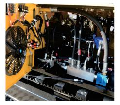
Utilizes a Sauer-Danfoss closed-loop piston pumps with merits of low energy consumption and high efficiency.
