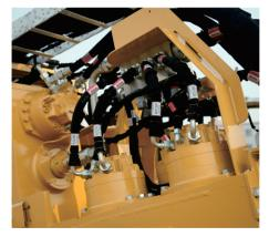
The imported Poclain drive motors maximize the efficiency of the system, saving energy and fuel, improving reliability and product life.
