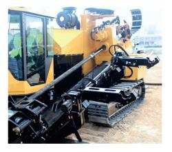
The standard setting includes high speed semi-auto rod stager with high speed carriage at 42m/min, enabling faster drill rod coupling improving work efficiency.
