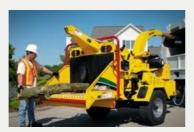
When there's tough brush-clearing work to do, you can count on the Vermeer BC1200XL to handle it. The electronic fuel injection engine provides improved fuel economy with 135 horsepower (101 kW). The PSI engine allows for more efficient working conditions and boosts engine response under load.
