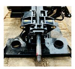
Open top vise design improves operator visibility when loading and unloading the drill rod. Vise logic can control and shut off the mud pump when the vise is closed. It also makes it easier to use the mud motors & other tooling.
